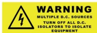
Example of sign required where multiple isolator / switch-disconnector devices are used
