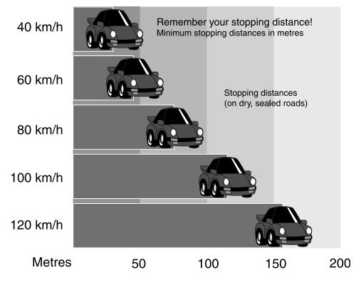
The following diagram indicates stopping distances for cars and light vans under ideal conditions on level ground.
