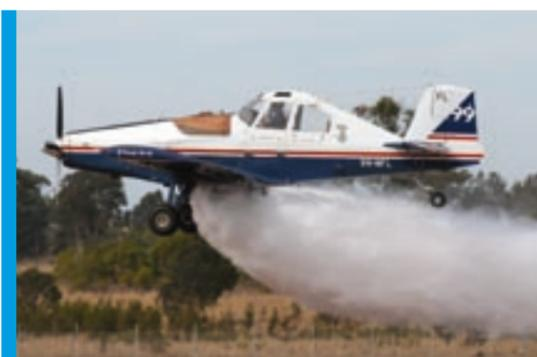
Ayres Thrush SR2 G10 uses Jet A1 fuel at the rate of 200 litres per hour, has a cruising speed of 240kph and carries 2,000 litres.
