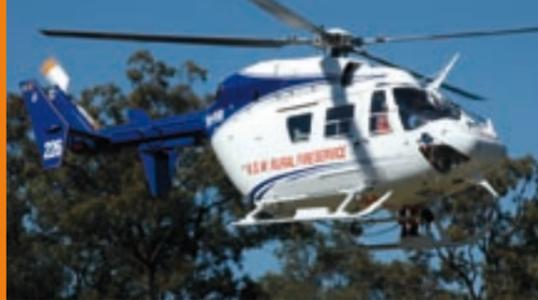
Kawasaki BK117 with twin engines and four blades, uses Jet A1 fuel at the rate of 300 litres per hour, has a cruising speed of 260kph and carries 1,100 litres.
