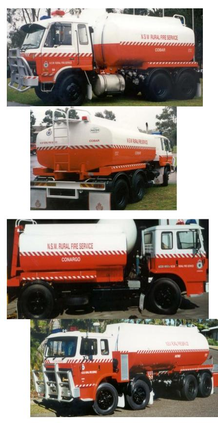
Brigade Name on Top of Lockers for all Tankers Cat 1 to 9 (indicative). (Note: Centre Locker forward of rear axle).
