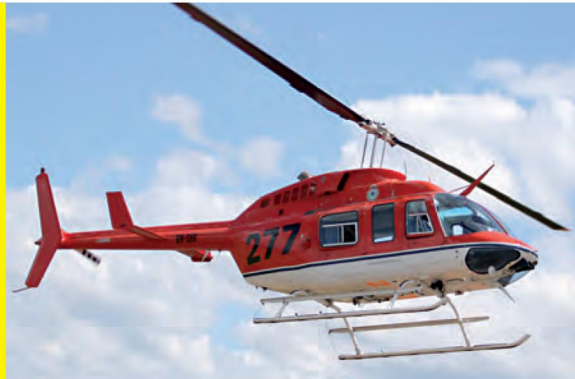
Bell 206L Long Ranger with one engine and 2 blades uses Jet A1 fuel at the rate of 170 litres per hour, has a cruising speed of 220kph and carries 680 litres.
