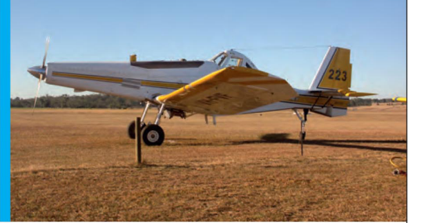
Turbine Dromader uses Jet A1 fuel at the rate of 260 litres per hour, has a cruising speed of 240kph and carries 2,500 litres.
