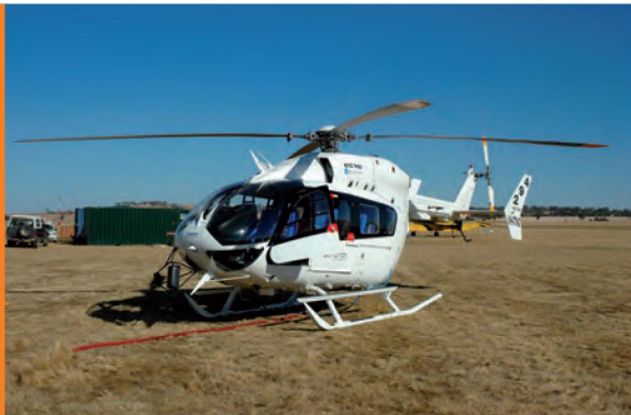
Eurocopter EC145 with twin engines and four blades, uses Jet A1 fuel at the rate of 300 litres per hour, has a cruising speed of 268kph and carries 1,100 litres.
