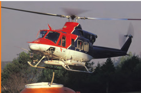
Bell 412 with twin engines and 4 blades, uses Jet A1 fuel at the rate of 380 litres per hour, has a cruising speed of 230kph and with belly-tank carries 1,420 litres.
