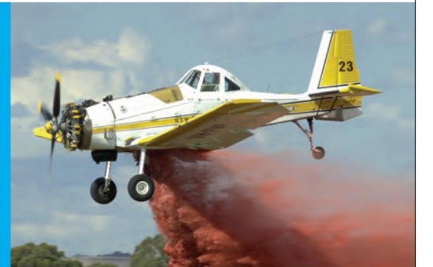
Radial Dromader, uses AVGAS fuel at the rate of 180 litres per hour, has a cruising speed of 200kph and carries 3,000 litres.
