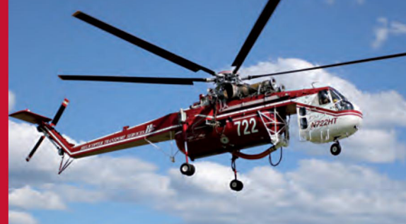
Sikorsky CH54B Sky Crane with twin engines and 6 blades, uses Jet A1 fuel at the rate of 2,080 litres per hour, has a maximum speed of 213kph and carries 9,000 litres.
