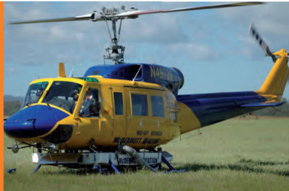
Bell 214B with single engine and 2 blades, uses Jet A1 fuel at the rate of 600 litres per hour, has a cruising speed of 260kph and with belly-tank carries 2,700 litres.
