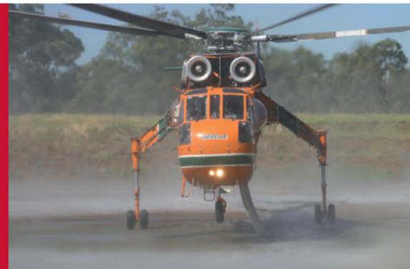
Erickson Air Crane S64 Series E (Isabelle) with twin engines and 6 blades, uses Jet A1 fuel at the rate of 2,080 litres per hour, has a max speed of 213kph and carries 9,000 litres.
