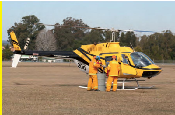
Bell 206 Jet Ranger with one engine and 2 blades, uses Jet A1 fuel at the rate of 105 litres per hour, has a cruising speed of 214kph and carries 455 litres.
