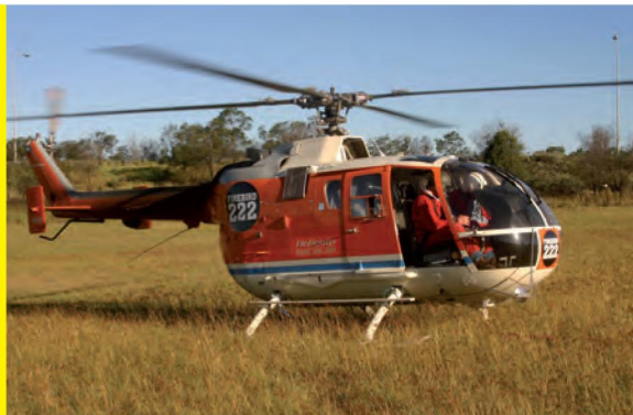
Eurocopter BO105 with twin engines and 4 blades, uses Jet A1 fuel at the rate of 250 litres per hour, has a cruising speed of 204kph and carries 800 litres.
