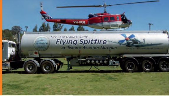
Bell 204 Restricted Category, with one engine and two blades, uses Jet A1 fuel at the rate of 320 litres per hour, has a cruising speed of 200kph and carries 1,500 litres.
