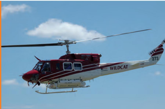
Bell 212 with twin engines and 2 blades, uses Jet A1 fuel at the rate of 360 litres per hour, has a cruising speed of 190kph and with belly-tank carries 1,300 litres.
