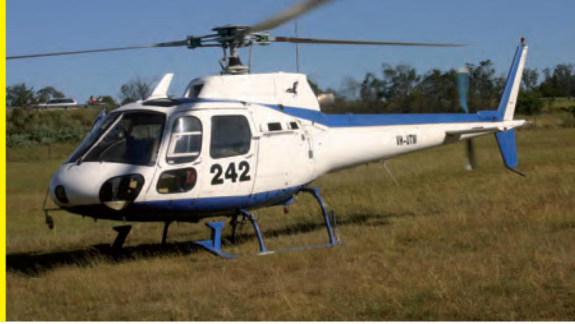
Squirrel AS350 with one engine and 3 blades, uses Jet A1 fuel at the rate of 170 litres per hour, has a cruising speed of 224kph and carries 680 litres.
