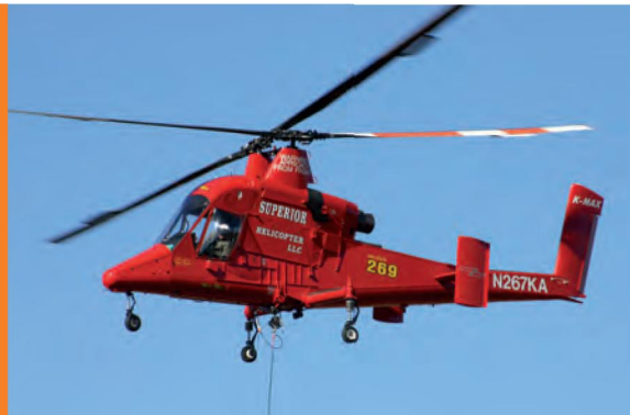
Kaman K-Max with single engine driving two side by side intermeshing, counter rotating blades, uses Jet A1 fuel at the rate of 310 litres per hour, has a maximum speed of 185kph and carries 3,000 litres.
