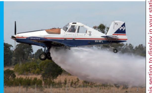
Ayres Thrush SR2 G10 uses Jet A1 fuel at the rate of 200 litres per hour, has a cruising speed of 240kph and carries 2,000 litres.
