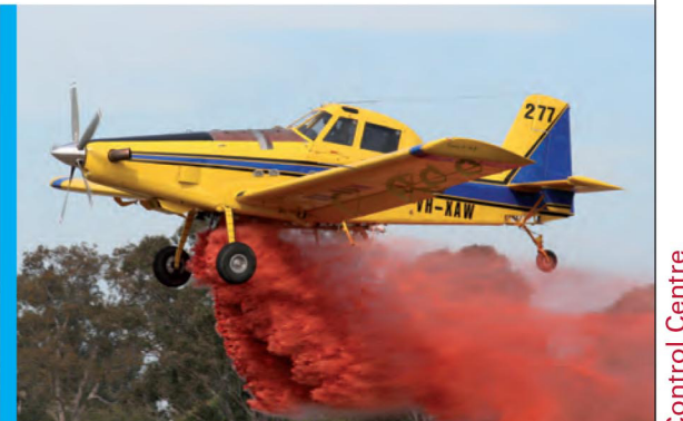
Air Tractor AT 802 uses Jet A1 fuel at the rate of 280 litres per hour, has a cruising speed of 280kph and carries 3,200 litres.
