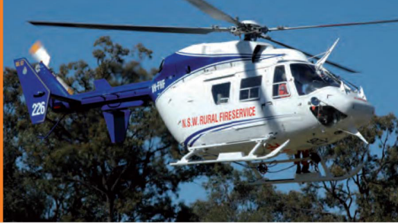
Kawasaki BK117 with twin engines and four blades, uses Jet A1 fuel at the rate of 300 litres per hour, has a cruising speed of 260kph and carries 1,100 litres.
