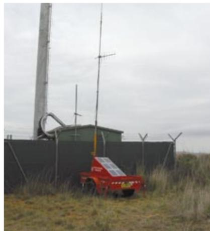
To ensure that reliable and robust communications are in place for volunteer firefighters this summer, the Canobolas Zone Portable Repeater was installed at the Clarkes Trig site to provide temporary network communications for operational communications pending installation of new hardware.
