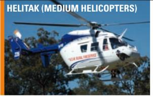
Kawasaki BK117 with twin engines and four blades, uses Jet A1 fuel at the rate of 300 litres per hour, has a cruising speed of 260kph and carries 1,100 litres.
