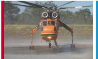
Erickson Air Crane S64 Series E (Isabelle) with twin engines and 6 blades, uses Jet A1 fuel at the rate of 2,080 litres per hour, has a max speed of 213kph and carries
