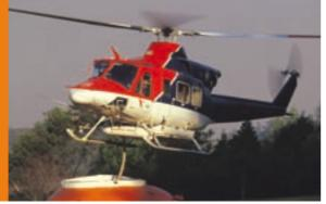
Bell 412 with twin engines and 4 blades, uses Jet A1 fuel at the rate of 380 litres per hour, has a cruising speed of 230kph and with belly-tank carries 1,420 litres.
