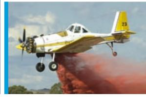
Radial Dromader, uses AVGAS fuel at the rate of 180 litres per hour, has a cruising speed of 200kph and carries 3,000 litres.
