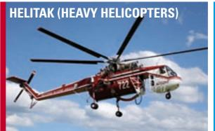
Sikorsky CH54B Sky Crane with twin engines and 6 blades, uses Jet A1 fuel at the rate of 2,080 litres per hour, has a maximum speed of 213kph and carries
