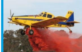
Air Tractor AT 802 uses Jet A1 fuel at the rate of 280 litres per hour, has a cruising speed of 280kph and carries 3,200 litres.
