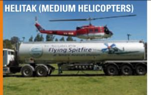
Bell 204 Restricted Category, with one engine and two blades, uses Jet A1 fuel at the rate of 320 litres per hour, has a cruising speed of 200kph and carries 1,500 litres.
