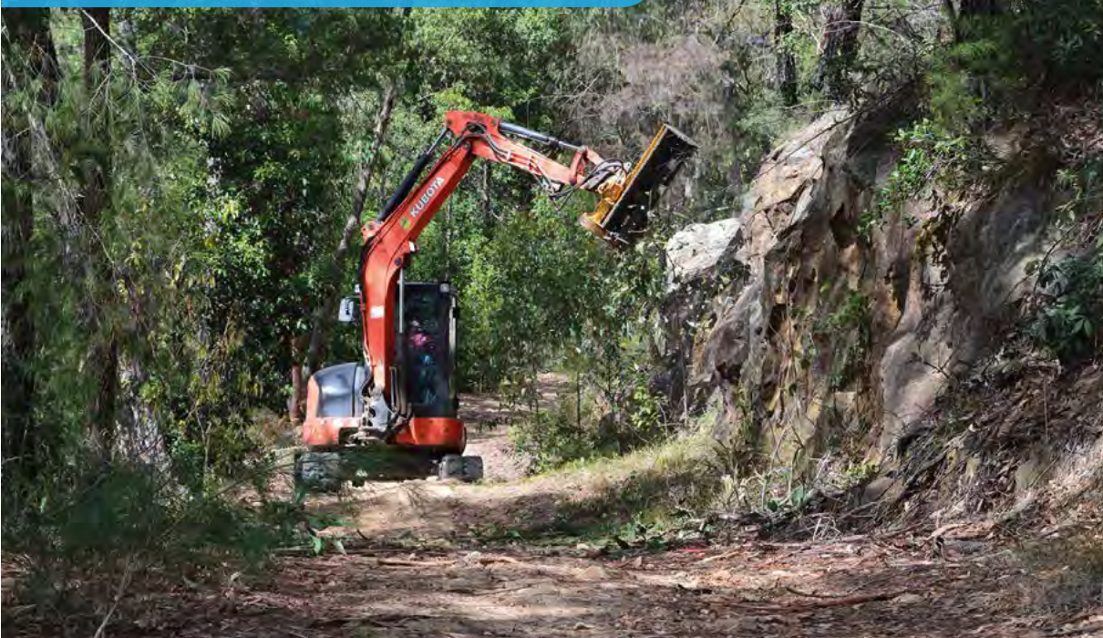
Photo 53 - An 8 t excavator with tritter mulching head is effective in managing vegetation.
