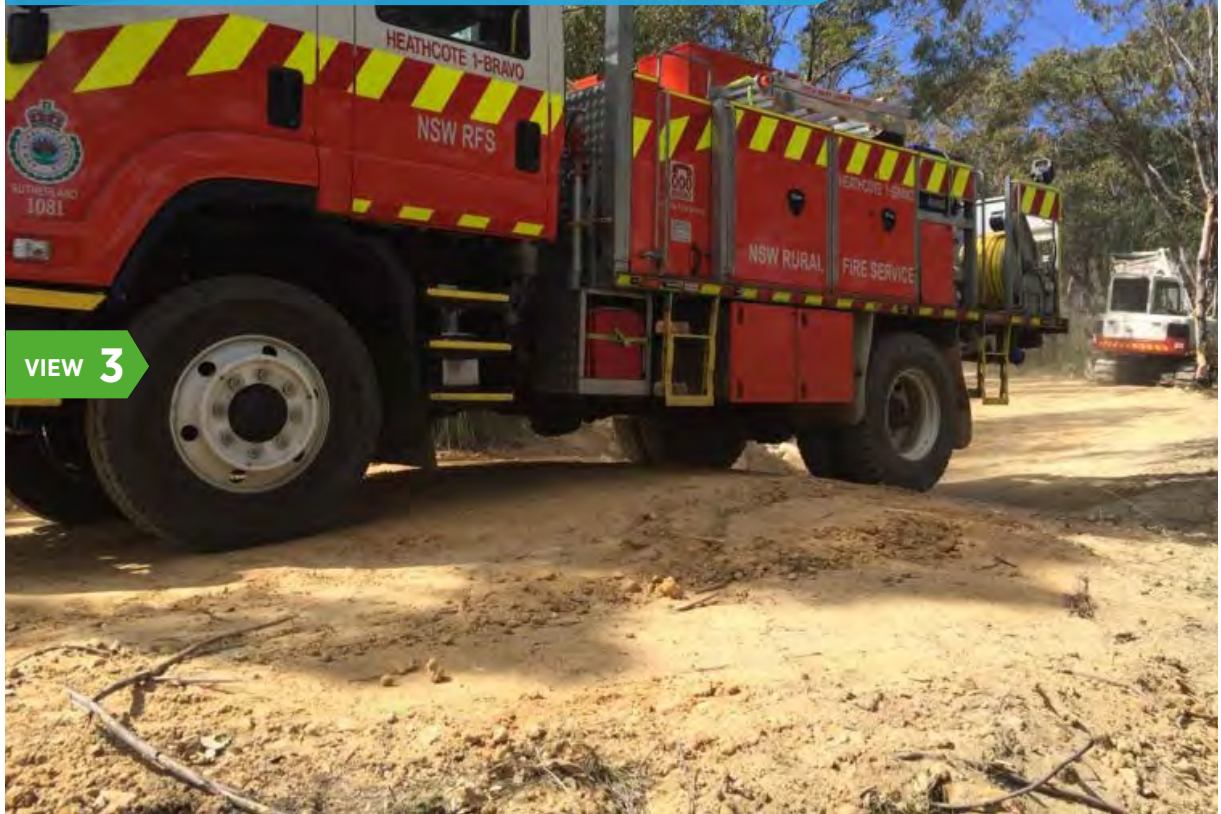
Photo 48 - Cross banks must be constructed so firefighting vehicles can clear without vehicle damage.
