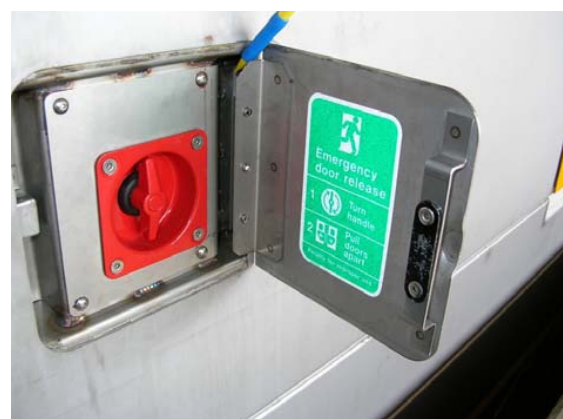
EEDR Turn handle clockwise to open door.
