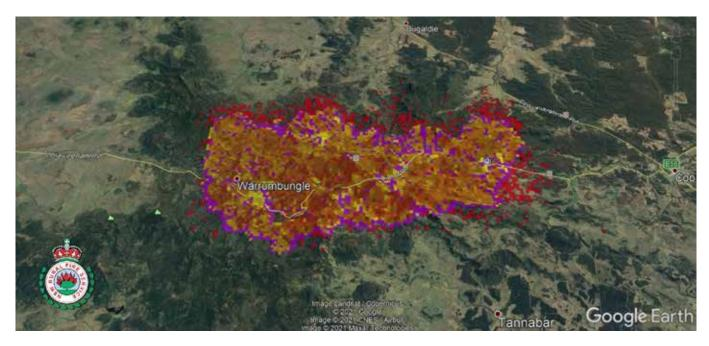
**Figure 3:** An example of a fire characterisation in PHOENIX RapidFire. The software predicts flame height (depicted in colours yellow and brown), ember attack (red) and locations where the fire edge will stop and extinguish (purple).
